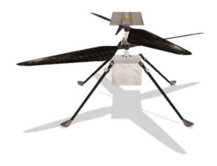
The Mars drone will be able to fly on it's own, without any human control and is expected to be able to fly for 90 seconds at a time!
